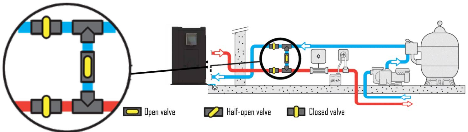
1. Unscrew the junctions to evacuate all the water contained in the HP.
