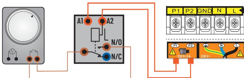
**Parameter for taking the connection into account:** Check that the setting of the filtration pump parameter (parameter #9) is set to "2". If this is not the case, please contact us to change the setting.
