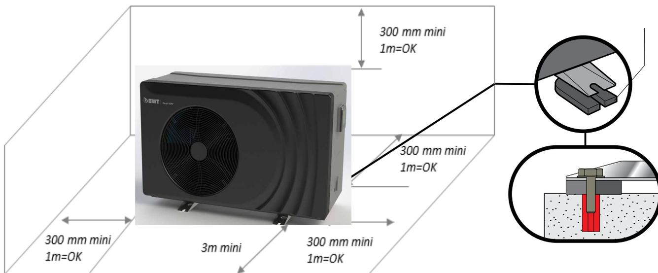
The HP must be installed and maintained on a fixed and solid basis, with the skids placed under the feet.
