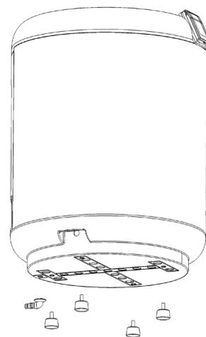
The HP must be installed and maintained on a fixed and solid basis, with the skids placed under the feet.
